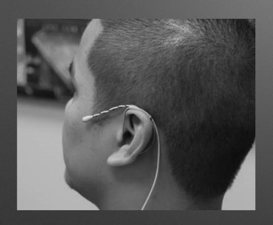
Mic attached to ear loop with Hellerman Sleeve, Heat Shrink, or just tape.
