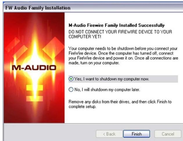
After the computer has been powered off, connect the FireWire SOLO to an available FireWire port on the computer and turn the FireWire SOLO power on. Once the FireWire SOLO is connected and powered, turn on your computer. Once Windows has fully loaded, the New Hardware Wizard will open. Choose the default selection, "Install the software automatically." Click "Next." Windows will locate and install the FireWire SOLO Bootloader files.
