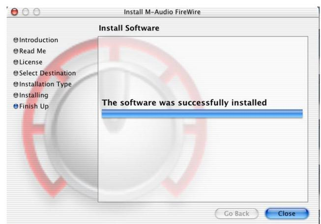
Once the installer has finished, you can shut down your computer. Plug the FireWire SOLO into your computer's FireWire Port. When the FireWire SOLO is connected, turn the computer back on. Once the operating system has loaded, go to "System Preferences" in the Apple Menu. Select the "Sound" preference panel, and click the "Output" tab. Select "M-Audio FireWire SOLO" to choose the FireWire SOLO as your default output device.
