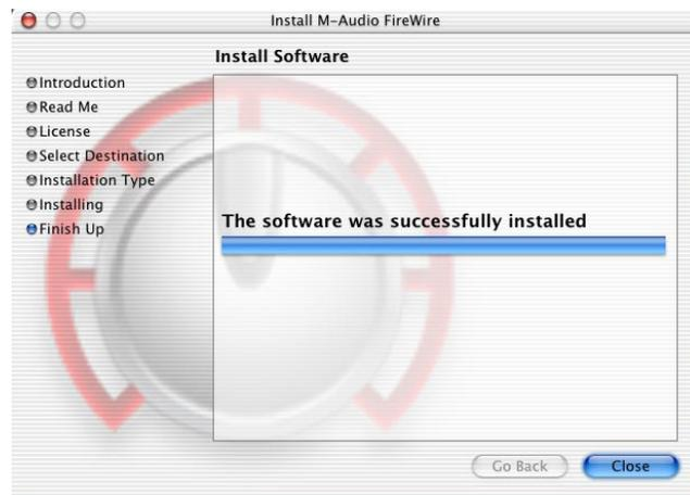
Once the installer is finished, you may shut down your computer. Plug the FireWire SOLO into your computer's FireWire Port. Once the FireWire SOLO is connected, turn the computer back on. Once the operating system has loaded, go to "System Preferences" in the Apple Menu. Select the "Sound" preference panel, and click the "Output" tab. Select "M-Audio FireWire SOLO" to choose the FireWire SOLO as your default output device.
