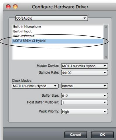
Figure 7-2: Enabling the 896mk3 Hybrid in Digital Performer
