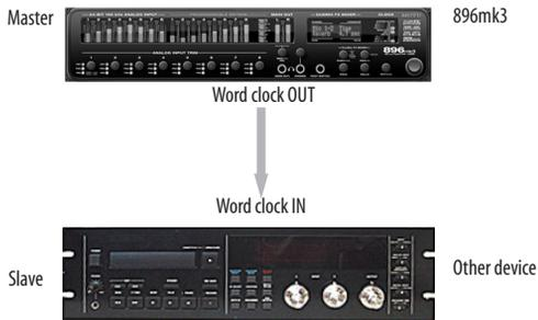
Figure 4-18: Slaving another digital audio device to the 896mk3 via word clock. For the 896mk3 clock source, choose any source besides word clock, as it is not advisable to chain word clock.
