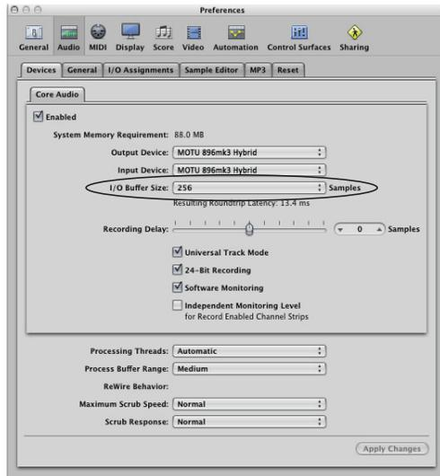
Figure 8-5: In Logic Pro or Logic Express, go to the Audio Devices preferences to access the Buffer Size option shown above.
