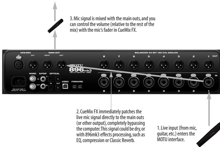
Figure 8-2: This diagram shows the signal flow when using *CueMix FX no-latency monitoring*. Notice that this method does not process the live input with plug-ins in your audio software. Instead, you can apply 896mk3 effects, such as the reverb, EQ and/or compression.
