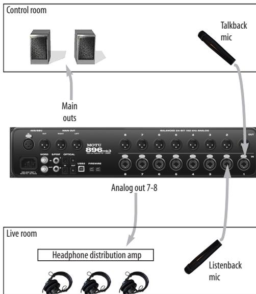
Figure 9-25: Typical hardware setup for Talkback and Listenback.
