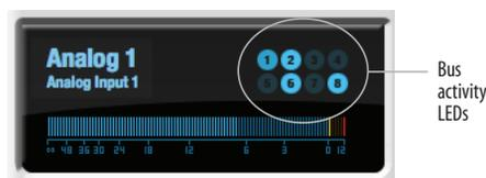
Figure 9-9: Input meter and bus activity LEDs.
