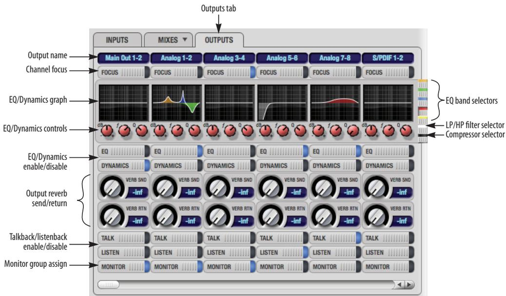
Figure 9-6: The Outputs tab.
