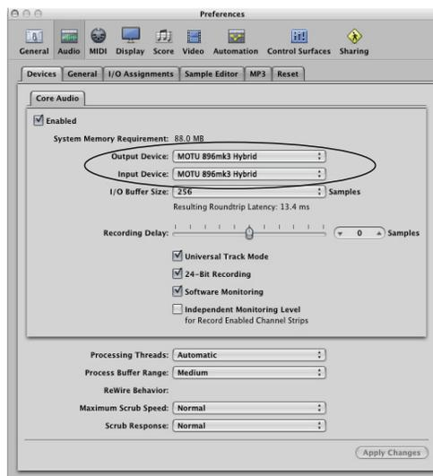
Figure 7-4: Enabling the 896mk3 Hybrid in Logic
