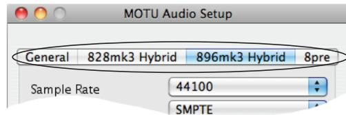
Figure 4-22: To view the settings for an interface, click its tab.
