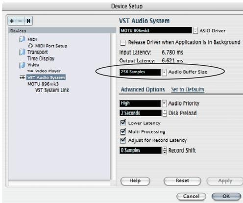
Figure 8-4: In Cubase or Nuendo, choose Devices menu > Device Setup. Select MOTU 896mk3 Hybrid, then click the Control Panel button to access the window above and the Buffer Size setting.
