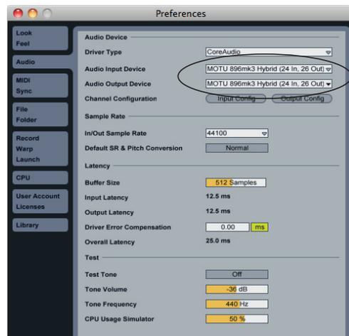
Figure 7-8: Enabling the 896mk3 Hybrid in Live
