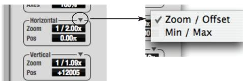
Figure 9-54: Setting the Horizontal or Vertical control modes.
