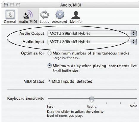
Figure 7-6: Enabling the 896mk3 Hybrid in Garage Band
