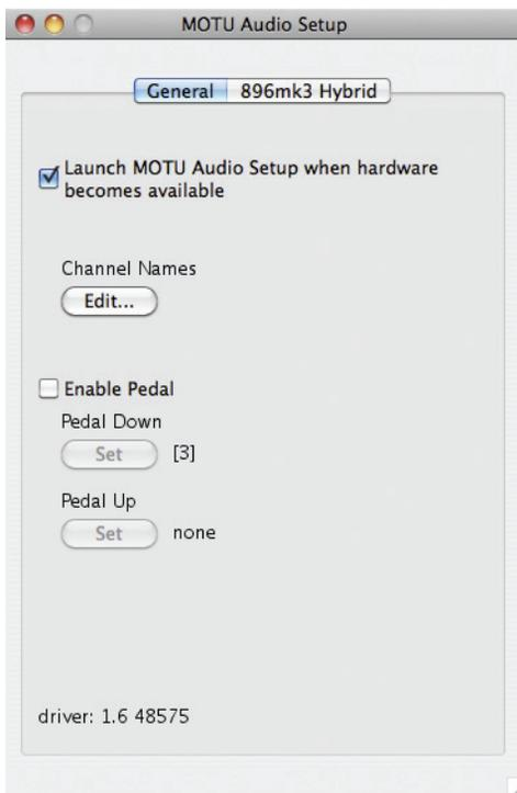
Figure 5-1: MOTU Audio Setup gives you access to all of the settings in the 896mk3 hardware.
