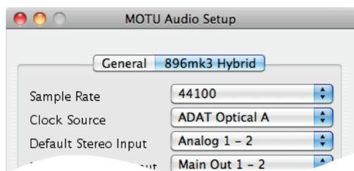
Figure 4-12: Resolving the 896mk3 to an optical device.
