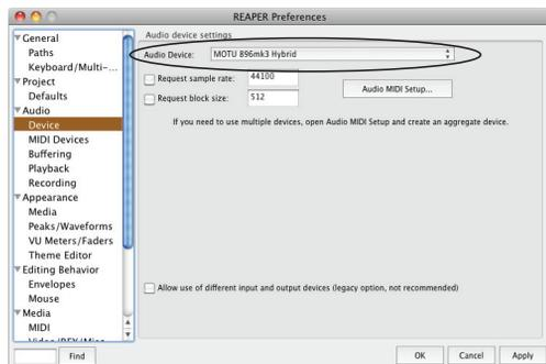
Figure 7-10: Enabling the 896mk3 Hybrid in Reaper
