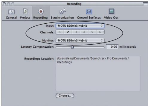
Figure 7-5: Enabling the 896mk3 Hybrid in Soundtrack Pro
