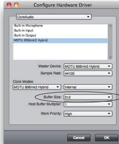
Figure 8-3: In *Digital Performer* and *AudioDesk*, choose *Setup menu > Configure Audio System > Configure Hardware Driver* to open the dialog shown above and access the *Buffer Size* setting. Refer to your *Digital Performer* or *AudioDesk* manual for information about the *Host Buffer Multiplier* setting.
