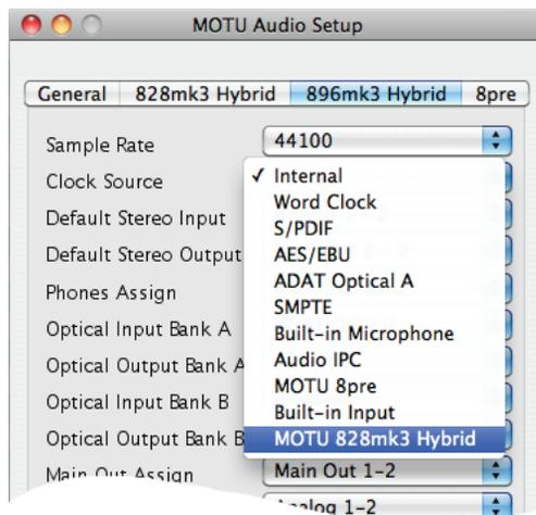
Figure 4-23: To resolve a MOTU interface to another Core Audio device, choose the other device from the Clock Source menu in MOTU Audio Setup. In this example, the 896mk3 will slave to the 828mk3.
