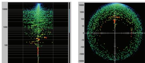
Figure 9-53: Rectangular versus Polar display with a logarithmic plot.
