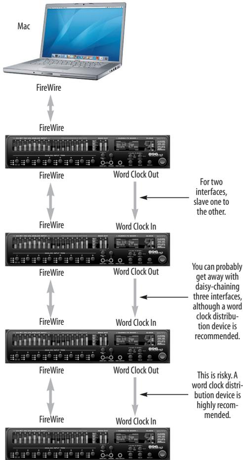
Figure 4-21: Connecting multiple 896mk3's (or other MOTU FireWire audio interfaces) to a computer.
