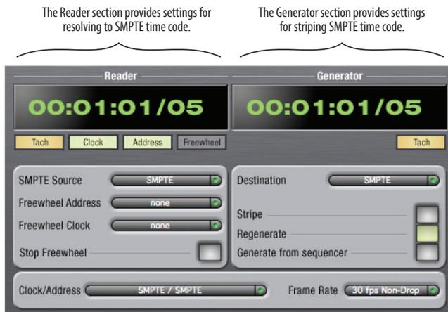
Figure 10-1: SMPTE Setup gives you access to your 896mk3's on-board SMPTE time code synchronization features.
