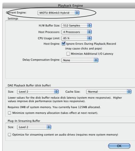
Figure 7-3: Enabling the 896mk3 Hybrid in Pro Tools
