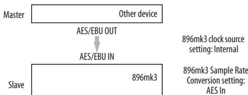
Figure 4-15: Rate-converting AES/EBU input.
