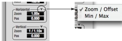
Figure 9-46: Setting the Horizontal or Vertical control modes.
