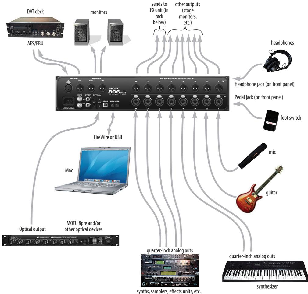
Figure 4-6: A typical 896mk3 studio setup.
