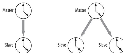
Figure 4-10: To keep the 896mk3 phased-locked with other digital audio devices connected to it, choose a clock master.
