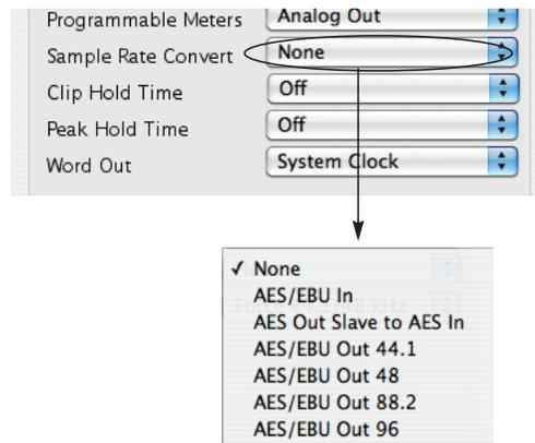
Figure 4-17: The Sample Rate Conversion option in MOTU Audio Setup gives you access the AES/EBU output clock options.
