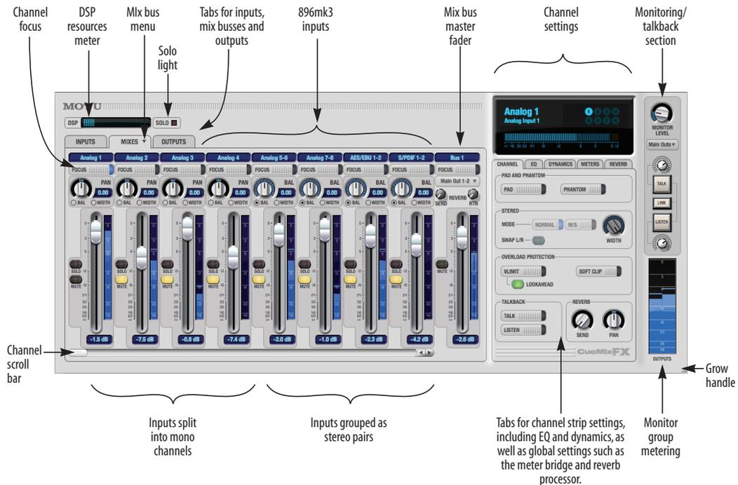
Figure 9-1: CueMix FX is a virtual mixer that gives you control over the 896mk3's on-board mixing features.
