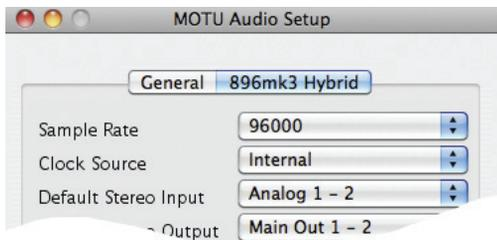
Figure 4-8: You can run the 896mk3 under its own internal clock when it has no digital audio connections and you are not synchronizing the 896mk3 system to an external time reference such as SMPTE time code.
