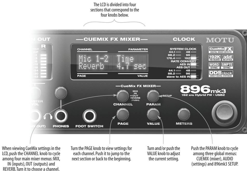
Figure 6-6: The 896mk3 Hybrid front panel controls.
